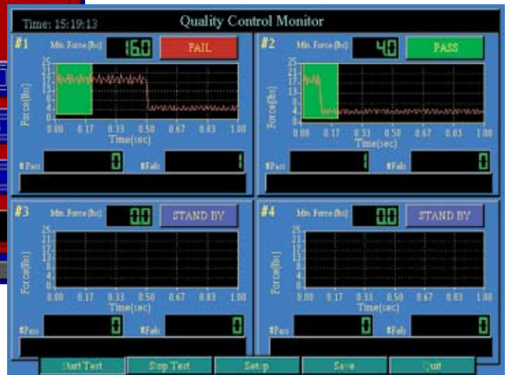
Screen showing IV Stopper Insertion Force versus Time Waveforms
