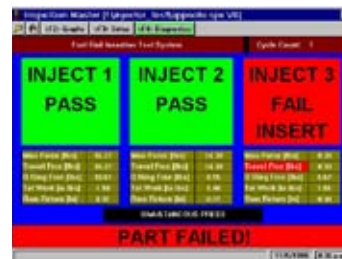
InspecXion Screen showing PASS/FAIL Messages Returned to Operator.
