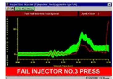
InspecXion Screen showing PASS/FAIL Signature Waveforms.
