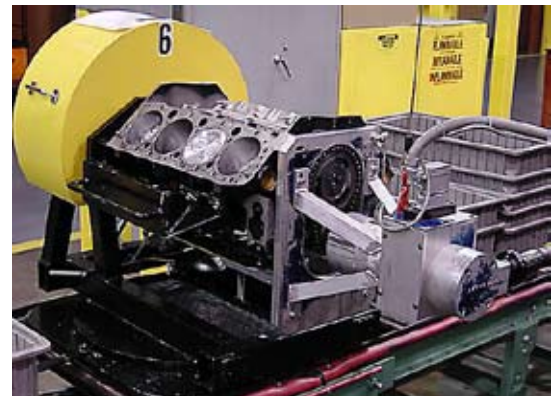
V8 Engine Block Test Station with metal test fixture mounted on front
