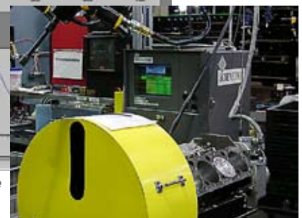
Side View of station showing Engine Block in foreground and Sciometric Test and Analysis System in background.
