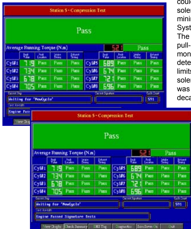
InSpeXion® Solenoid Assembly Screens showing Test Diagnostics.
